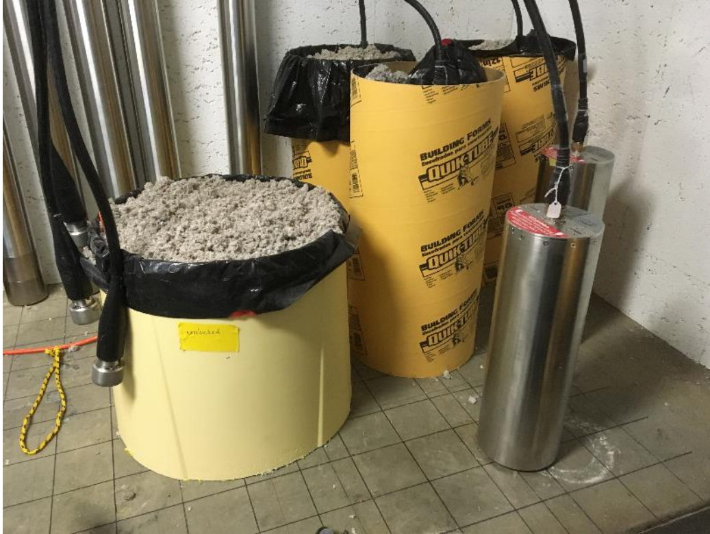
Figure 3 Picture of installed seismometers, before insulation
