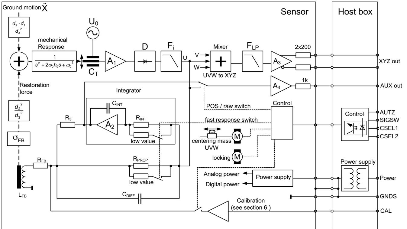
The block diagram shows only the component U. V and W are identical and omitted for simplicity.
