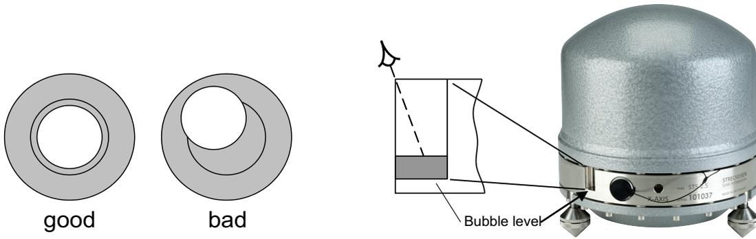
**!** Finally tighten all three feet by turning their counter nuts clockwise until they lock firmly. Check it. A loose foot will strongly compromise the signal quality.
