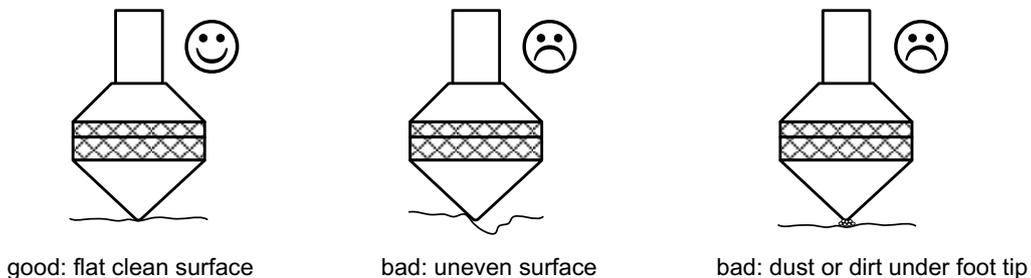
Avoid areas where corrosive inclusions such as iron are near or directly under the feet tips. Corrosive processes are most prominent on the horizontal components. Cementing small glass plates (50x50x5mm) with slow hardening cement (free of sand) as foot rest have been proven very effective. Avoid trapped air bubbles during cementing process.
